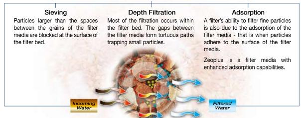
Micron W series filter is capable of filtering out particles as small as 10 microns (0.01mm).
